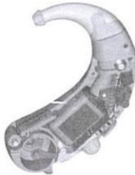
Fig. 1.3 A digital hearing aid employing signal processing technique (Siemens TRIANO 3 Digital hearing aid; Siemens Audiology Copyright© 2005)
