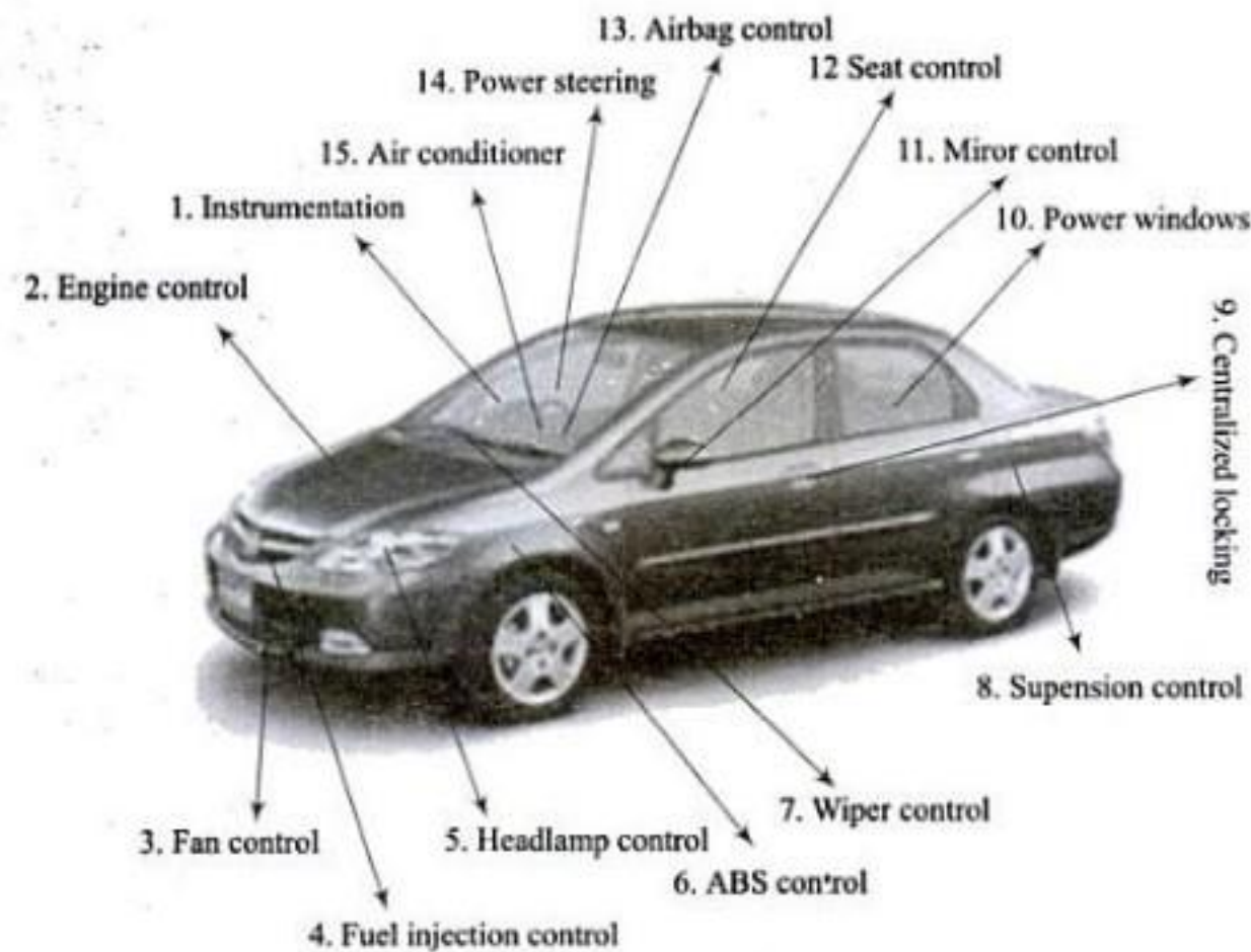
Fig. 4.3 Embedded system in the automotive domain (Photo courtesy of Honda Siel Car India ( www.hondacarindia.com ))
